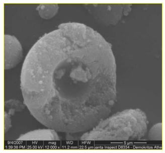
Figure 7b: **SEM images of hollow silica microspheres with porous shells** – Procedure A
