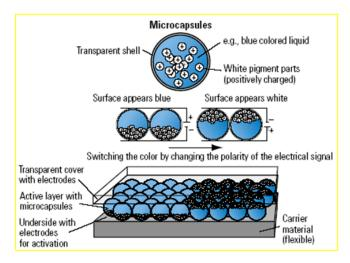
Figure 2: Schematic representation of the principle of operation of the e-ink. Source: E Ink – Phillips Research.
