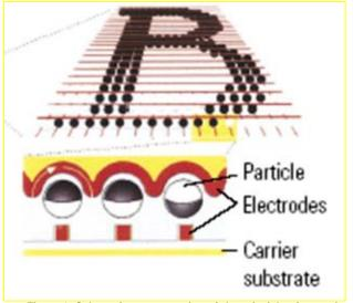
Figure 1: Schematic representation of the principle of operation of the Gyricon beads e-paper. Source: Xerox Corporation.
