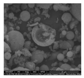
Figure 7a: SEM images of hollow silica microspheres with porous shells – Procedure A
