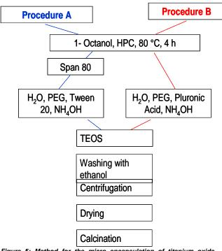
Figure 5: Method for the micro encapsulation of titanium oxide particles for use in e-paper applications.
