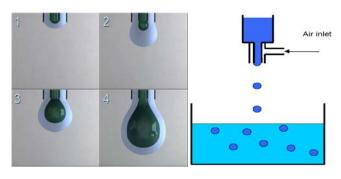
Figure 6: Experimental arrangement for the development of silica microcapsules for e-paper applications
